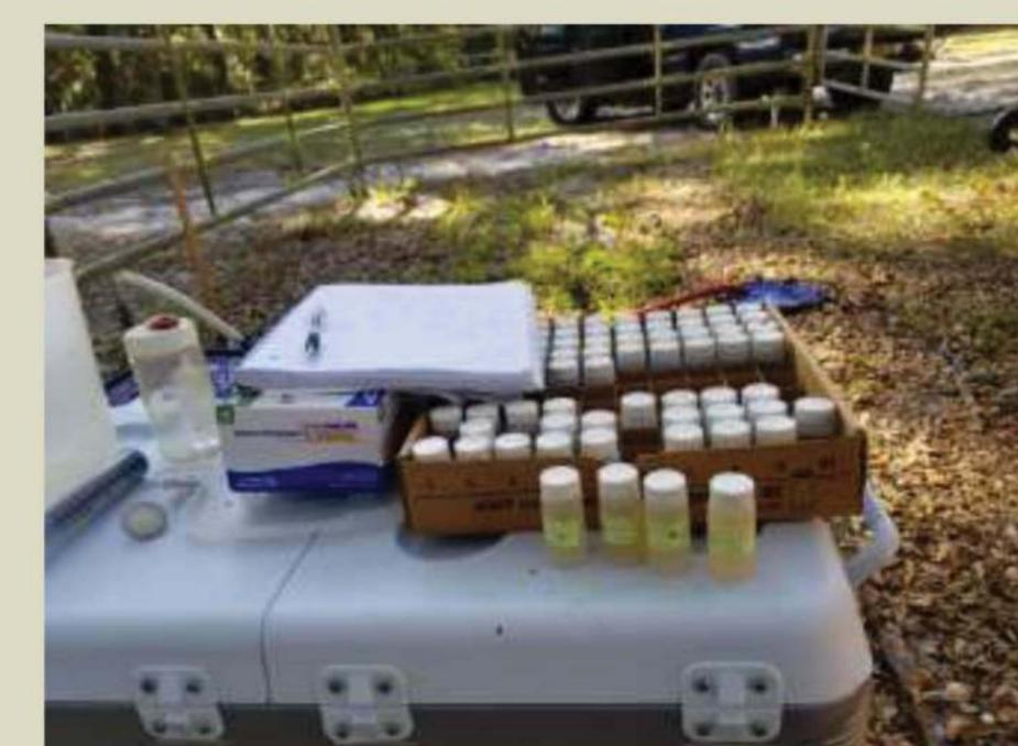
Water samples are obtained from each site with below ground lysimeters, then the samples are analyzed to characterize nutrients.
